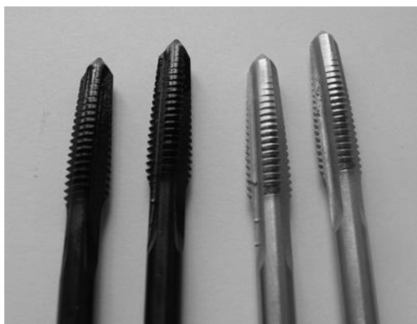
Figure 2. Taps M6 without processing and with chromium coating
