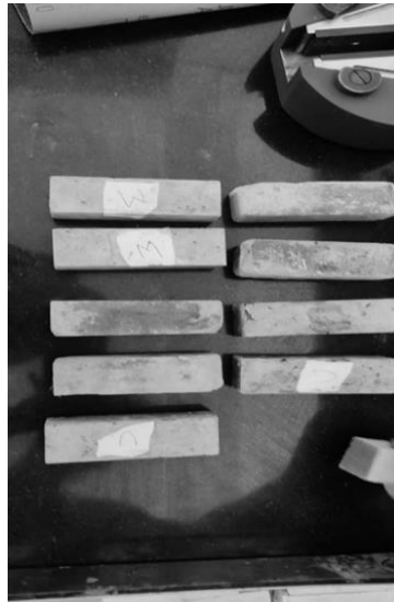
Figure 4. Casted beams after curing
