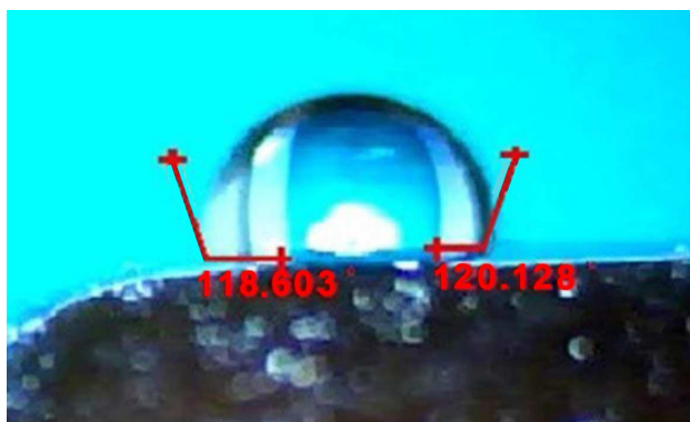
Figure 11. A water droplet on the surface of a coated outdoor insulator after working in an air atmosphere under sunlight for sixty days (contact angle is about 120°)
