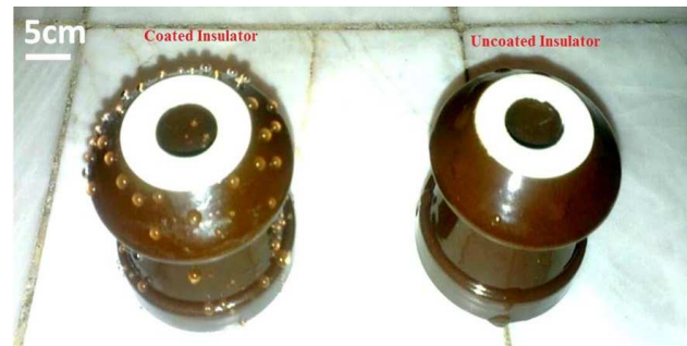
Figure 10. The uncoated and coated outdoor insulators
