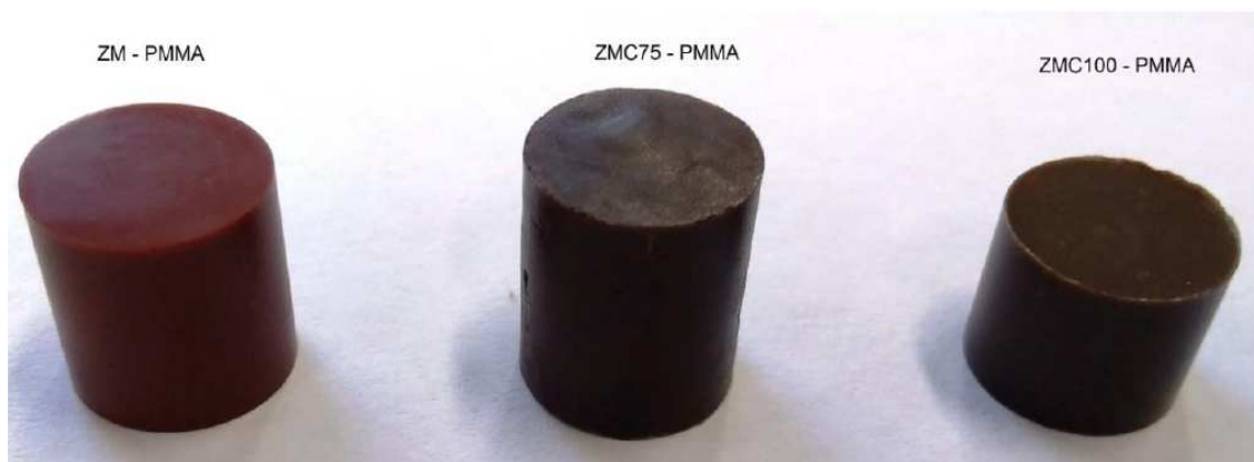
Figure 8. PMMA samples coloured with ZM and ZMC pigments
